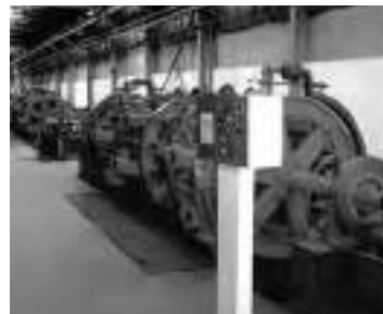
6+12+18 Planetary Strander for non-rotational Crane Ropes
