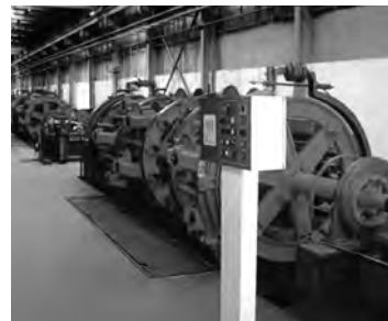
6+12+18 Planetary Strander for non-rotational Crane Ropes
