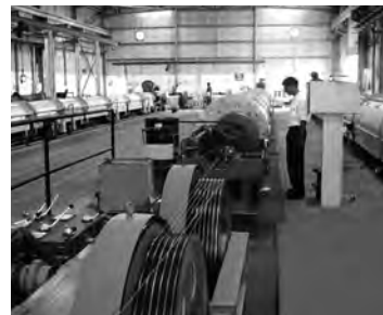
Wire Spooling & Long Stranding Machines (18 Bobbin, 25 Bobbin & 3 no. 36 Bobbin)
